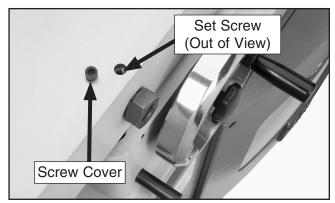
Figure 51. Screw cover and set screw location.
